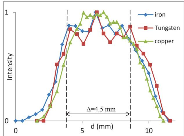
Figure 3: Peak intensity as a function of sample displacement for Fe, W and Cu defects.
