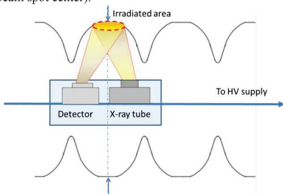
Figure 4: Draft of XRF probe.
