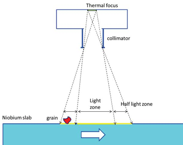
Figure 2: set-up arrangement for lateral sample scanning
