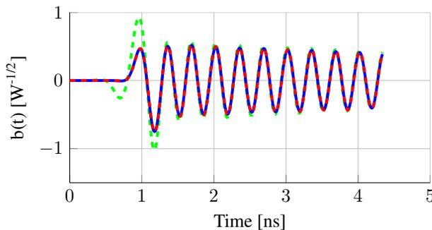
Figure 3: Transient signals at port 1 excited by a beam with  $q = 1 \text{ nC}$  and  $\sigma = 35 \text{ mm}$ , with no shift from default position.
