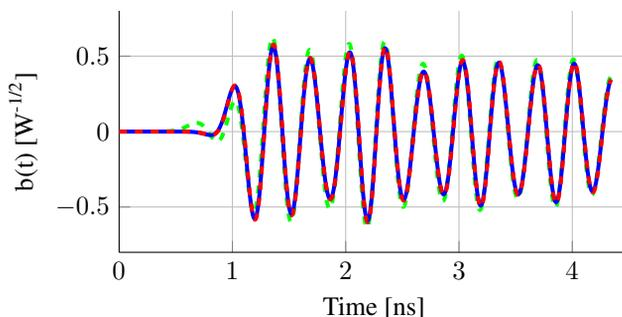
Figure 4: Transient signals at port 3 excited by a beam with  $q = 1 \text{ nC}$  and  $\sigma = 35 \text{ mm}$ , with shift of  $x_0 = 3.1415 \text{ mm}$  and  $y_0 = -14.03 \text{ mm}$  from default position.
