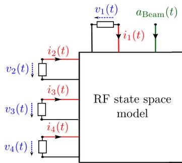
Figure 2: Equivalent circuit with modal voltages (in red), modal currents (in blue) and incident beam power (in green) and the impedances of the couplers as port impedances of  $50 \Omega$ .
