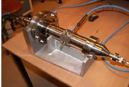
Figure 3 Test bench for BPM block
