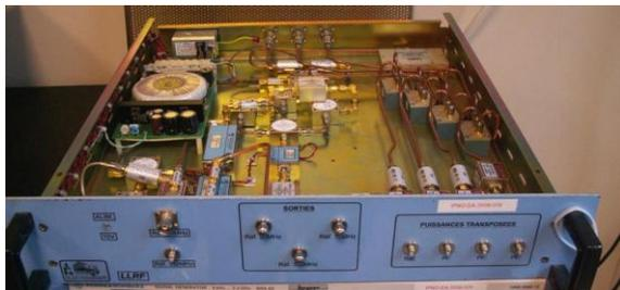
Figure 5 V1 Down converters system
