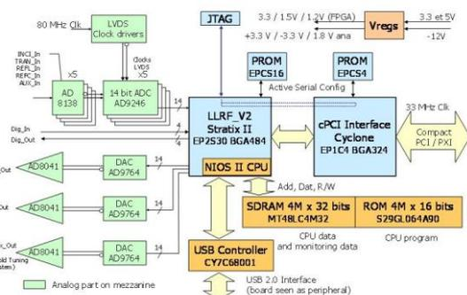
Figure 4 V2 board block diagram
