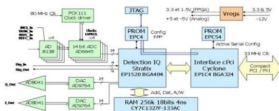
Figure 2 V1 board block diagram
