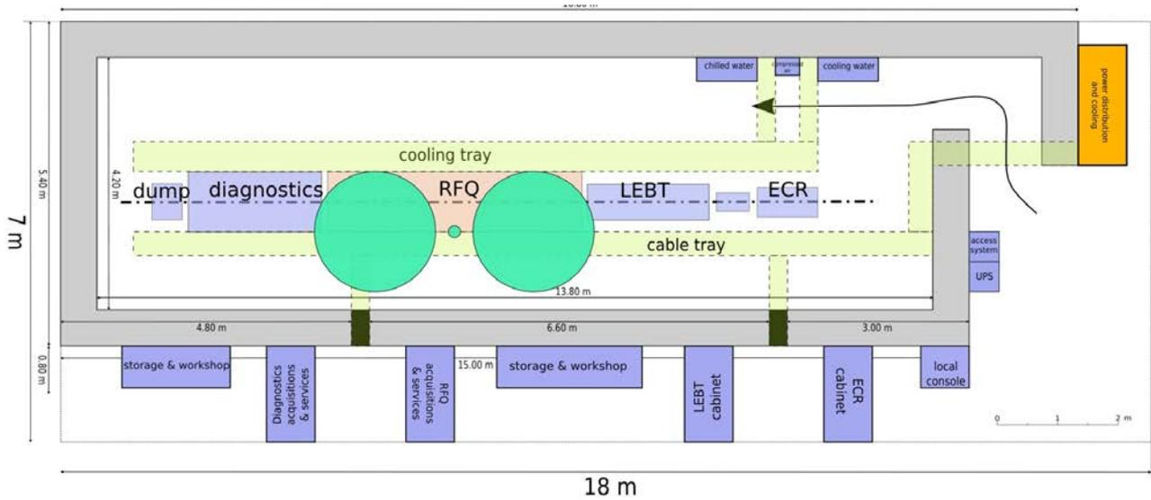
Figure 3: General layout of the experimental setup of RFQ@UCL R&D program
