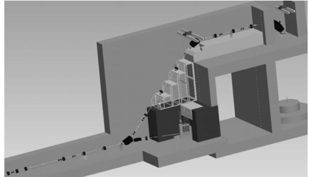
Fig. 5. Layout of the MYRRHA beam lines to reactor and dump (courtesy of H. Saugnac).
