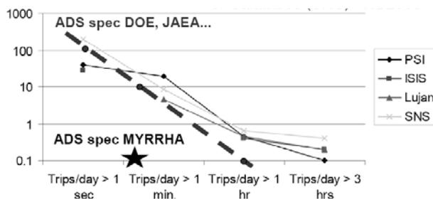
Fig. 1. Trip frequency vs. trip duration for high power proton accelerators<sup>16</sup> & ADS specifications.
