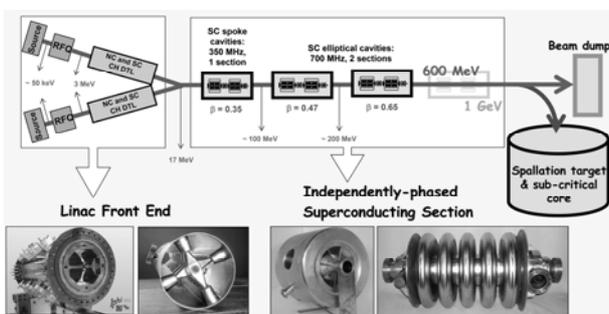
Fig. 2. Conceptual scheme of the MYRRHA accelerator.
