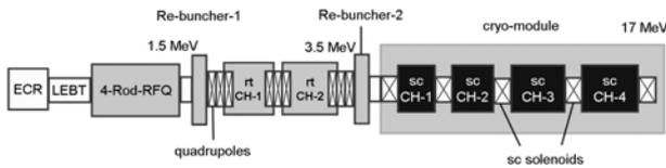
Fig. 3. Schematic overview of the 176 MHz injector (courtesy of H. Podlech and C. Zhang).
