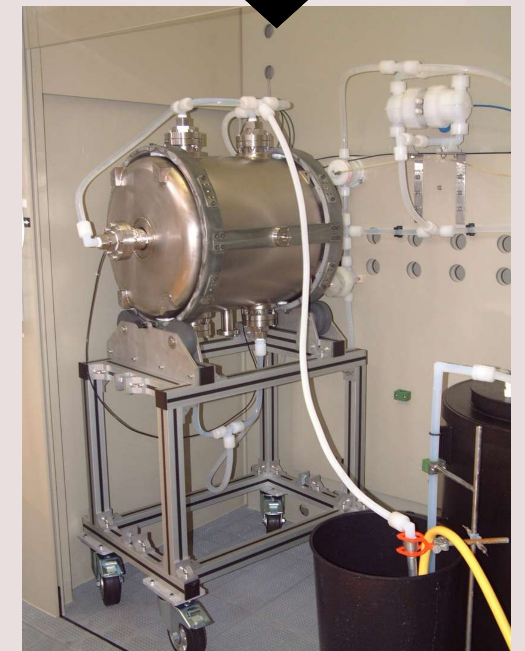
The cavity is rinsed with ultra- pure water
