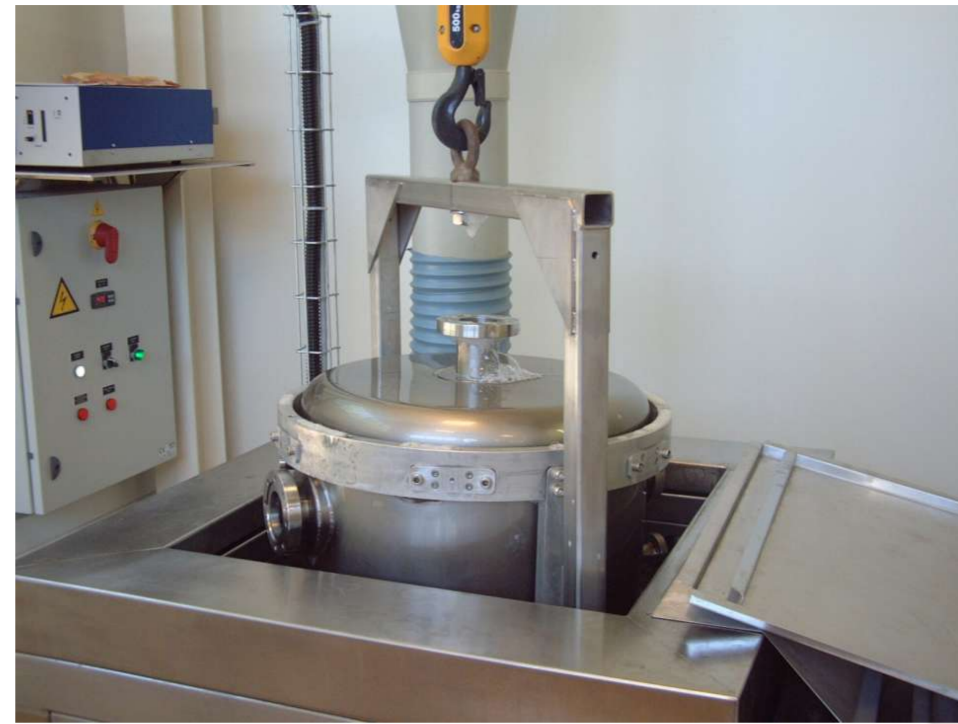
The cavity is then degreased in a ultrasonic bath
